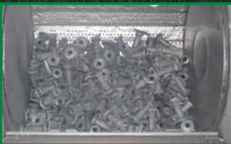
Smaller castings are tumble blasted and cleaned with a Pangborn Roto-Blast.
