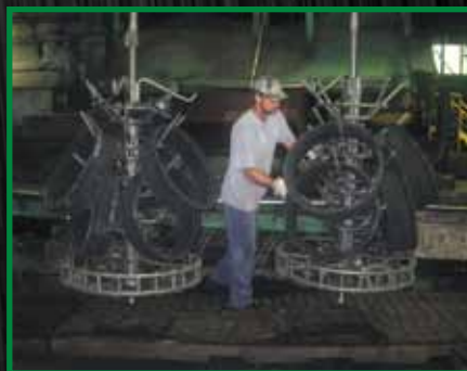
Larger castings are hung on trees and sent through cabinet blaster for cleaning.
