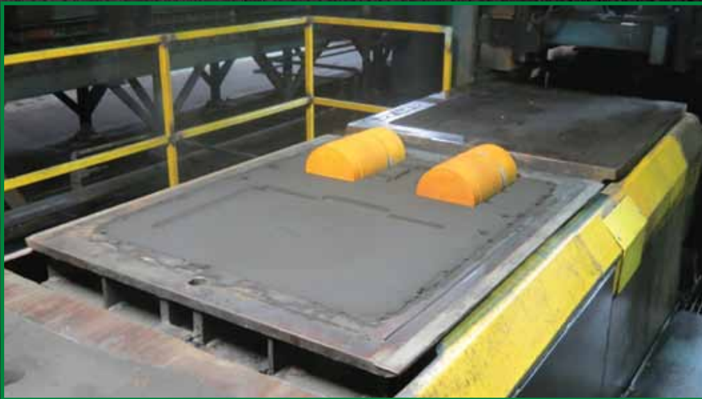
Both cored and no-cored castings are available on the Herman Mold Master. Flask size of 34" x 44" allows a wide variety of castings configurations and combinations.
