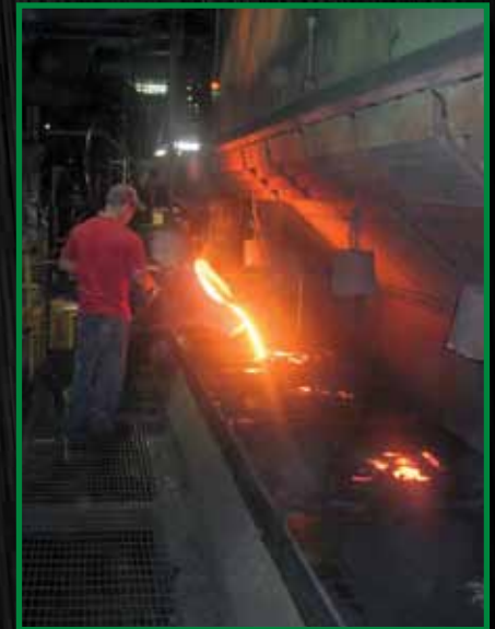
The Herman Mold Master offers dimensional accuracy combined with a quality finish. Multiple impression molds or castings weighing 350 lbs. can be produced on the Mold Master.
